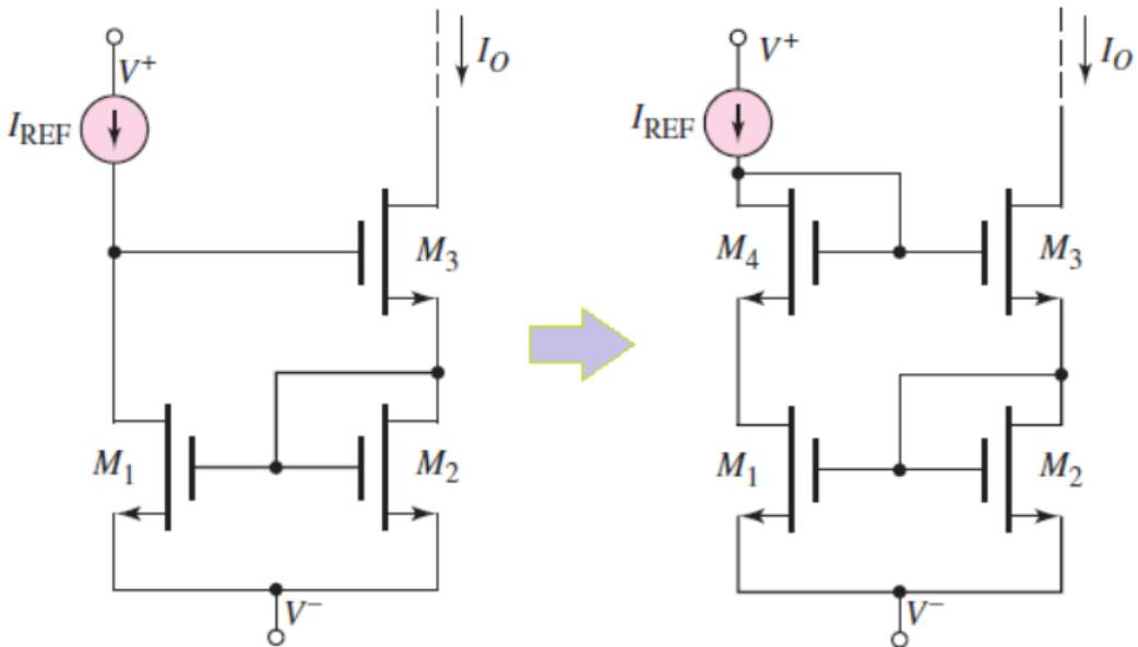
Since  $\lambda$  is not zero, the ratio  $\frac{I_O}{I_{REF}}$  is slightly different from the aspect ratios. This problem is solved in the **modified Wilson current source**
