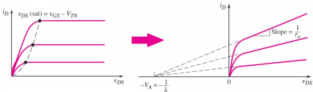
$$I_D = \frac{1}{2} K_n V_{OV}^2 (1 + \lambda V_{DS})$$
