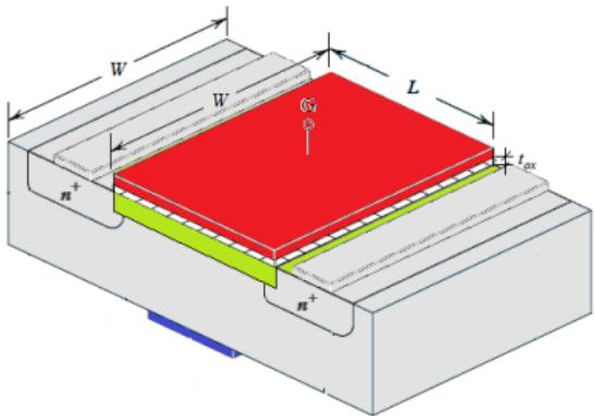
$t_{ox}$  of  $0.13\mu m$  technology = 2.7 nm, 45nm technology = 1.4 nm.
