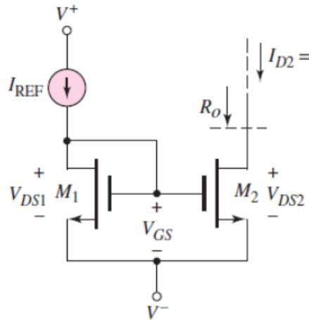
$$I_o = 0.5K_{n2}(V_{GS} - V_{TN2})^2$$
