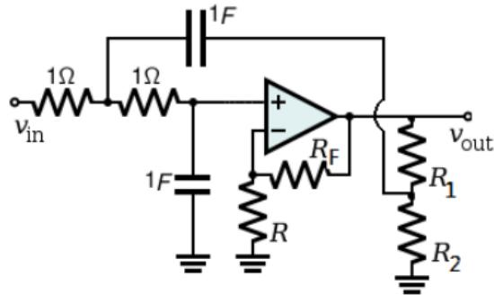
$$T(S) = \frac{k \frac{1}{R_1 R_2 C_3 C_4}}{S^2 + [\frac{1}{R_1 C_3} + \frac{1}{R_2 C_3} + \frac{1}{R_2 C_4} - \frac{k k_d}{R_2 C_4}] S + \frac{1}{R_1 R_2 C_3 C_4}}$$
