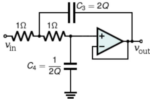
$$T(S) = \frac{k \frac{1}{R_1 R_2 C_3 C_4}}{S^2 + [\frac{1}{R_1 C_3} + \frac{1}{R_2 C_3} + \frac{1}{R_2 C_4} - \frac{k}{R_2 C_4}]S + \frac{1}{R_1 R_2 C_3 C_4}}$$
