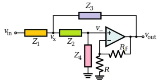
$$\frac{V_{out}}{V_{in}} = \frac{KZ_3Z_4}{Z_1Z_3 + Z_1Z_2 + Z_2Z_3 + Z_1Z_4 + Z_3Z_4 - KZ_1Z_4}$$
