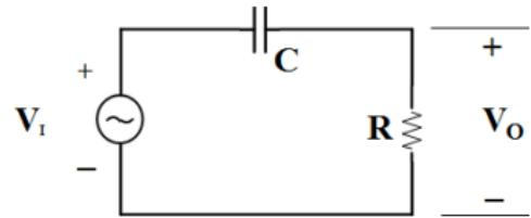
$$|T(S)| = \frac{\frac{\omega}{\omega_c}}{\sqrt{1 + (\frac{\omega}{\omega_c})^2}}$$
