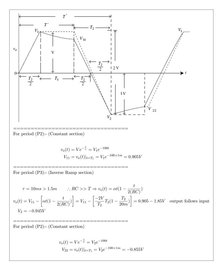
3. The input signal shown in next figure is applied to a RC high-pass circuit, whose time constant is 0.4 ms. Draw the output waveform and mark all voltages, assuming that the capacitor is initially uncharged.  $[10 \text{ marks}] [D_c]$
