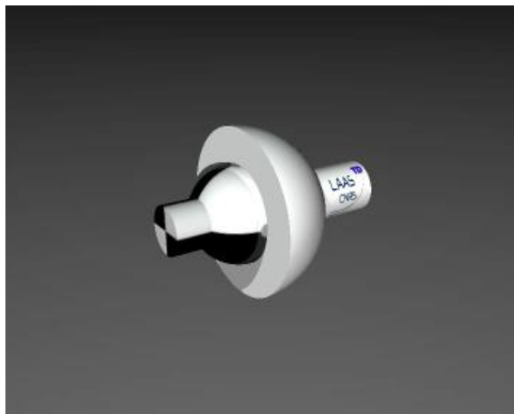
Spherical (S) joint—3 DOF
