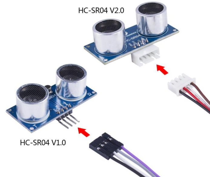
Anti-reverse port(JST-XH) for HC-SR04 V2.0
